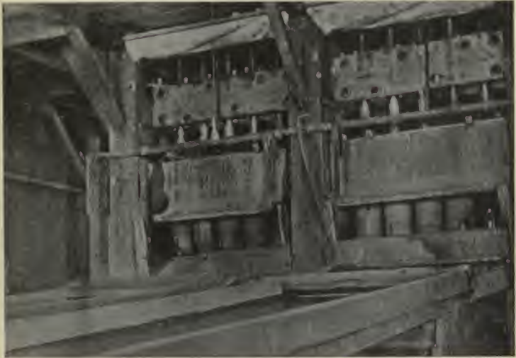
· FIG. 103.—THE STAMPS IN A QUARTZ-MILL
